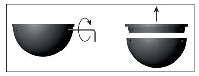
4. Screw the arms to the half-sphere. The curved part of the arms has to be parallel to the ceiling and in the alignement of the half-sphere. Screw strongly the nuts in the half-sphere to avoid unscrewing.
